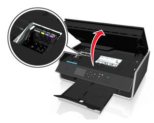
**Note:** The printhead moves to the cartridge installation position.
